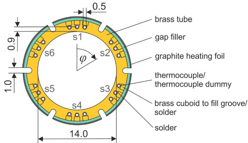
Fig. 2. Cross-sectional view of test section at a plane of measurement. The thermocouples in the plane of measurement 1, pm1, are located at angles  $\varphi = 0^\circ; 60^\circ; 120^\circ; 180^\circ; 240^\circ; 300^\circ$ . The angle is measured mathematically negative due to historical reasons.
